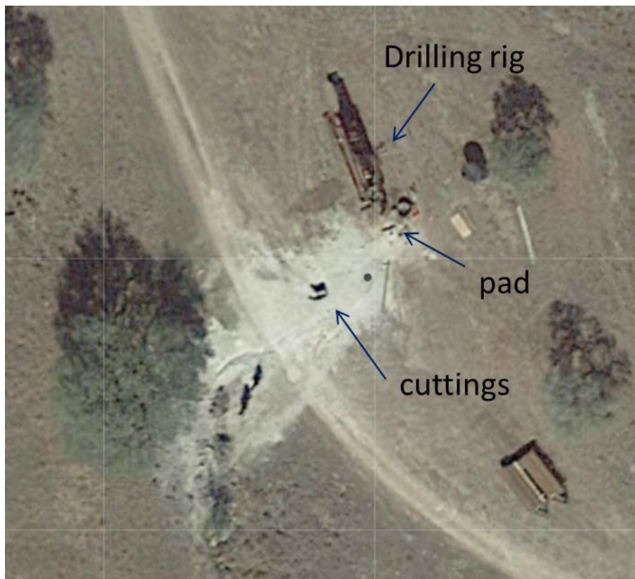
Figure 5. Drilling rig for the Blue Pine Holdings well drilled from Nov. 2016 to Jan 2017 shows the rig, drill pad and cuttings.
