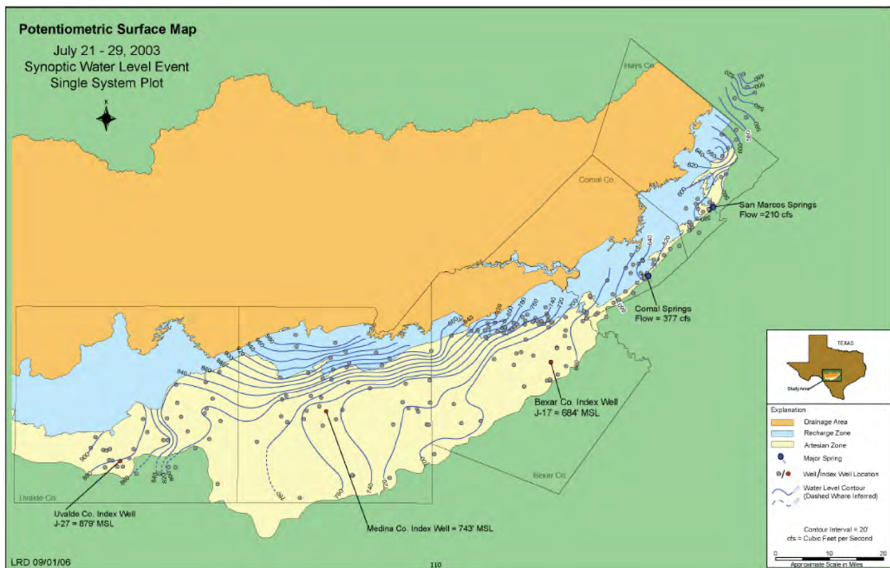
Figure 8. Potentiometric surface map showing approximate Edwards groundwater flow direction in south-central Comal County to be to the southeast (Johnson et al., 2006).
